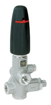
GENERAL PUMP UNLOADER 316SS -1/2BSP-F - MAX 7250PSI -MAX 16 GPM
