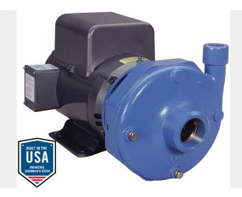
IRON/BRONZE | BUNA MECH SEAL | 3 HP TEFC, 3500RPM, 1/60/230 VOLTS | 1.5 X 2-6 | BEP 89 GPM @ 98FTH
