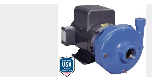
ALL BRONZE | BUNA MECH SEAL | 5 HP TEFC, 3500RPM, 1/60/230 VOLTS | 2.5X 3-7 | BEP 171 GPM @ 65FTH | Product photo could vary from the actual product
