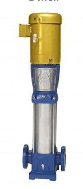
Wetted Parts: Cast Iron, 304SS, Viton Seal | 3 Phase | 10 hp | 3600 rpm | 2" Flanges | BEP 45 GPM @ 550 FTH | **PREM. EFF. MOTOR**
