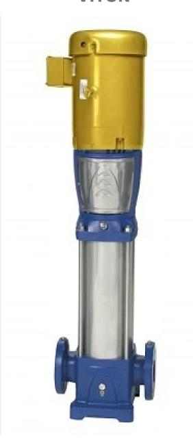
Wetted Parts: Cast Iron, 304SS, Viton Seal | 3 Phase | 1.5 hp | 3600 rpm | 1.25" Flanges | BEP 9 GPM @ 260 FTH | **PREM. EFF. MOTOR**
