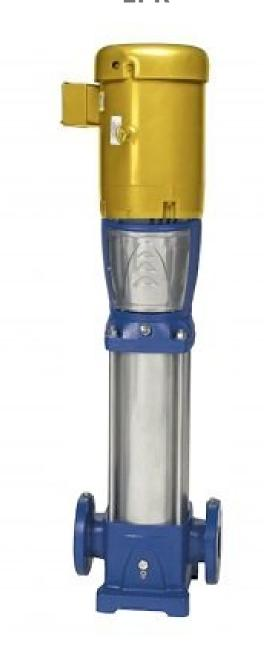
Wetted Parts: Cast Iron, 304SS, EPR Seal | 3 Phase | .5 hp | 3600 rpm | 1.25" Flanges | BEP 9 GPM @ 95 FTH | **PREM. EFF. MOTOR**
