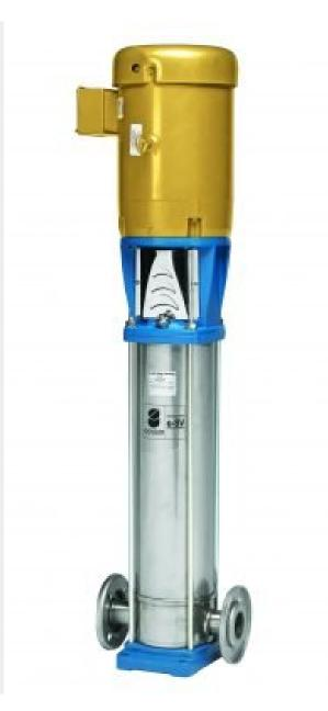
Wetted Parts: 304SS, Viton Seal | 3 Phase | 5 hp | 3600 rpm | 2" Flanges | BEP 100 GPM @ 110 FTH
