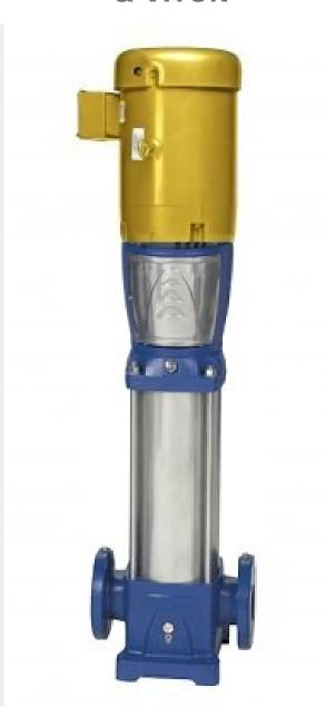
Wetted Parts: Cast Iron, 304SS, Viton Seal | 7.5HP | 3Phase | TEFC | 3500 rpm | 1.25" Flanges | BEP 30 GPM @610 FTH
