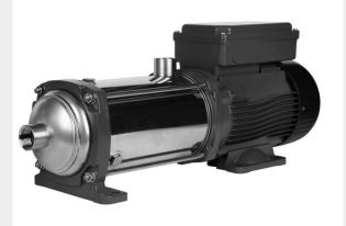
BEP 45 GPM @ 180 FTH | Wetted Material 316SS & Car/Silcar EPDM or Viton | 60 Hertz 208-230/460V / 50 Hertz 220-240/380-415V | 1.50"NPT
