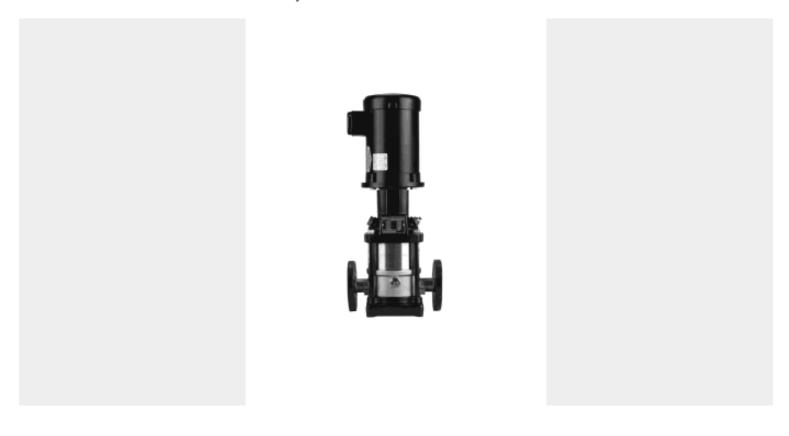
96522974 Wetted Parts: 316SS, Viton Seal | 1 Phase | 10 hp | 3600 rpm | 2" Flange 300lb | BEP 45 GPM @ 510 FTH
