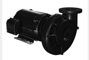
CAST IRON/STAINLESS IMPELLER | BUNA MECH SEAL | 15HP TEFC PRE EFF, 3600RPM, 3/60/208/230-460 VOLTS | 2.5 X 2 - IMPELLER 6.29" | CONNECTIONS- NPS | BEP 250 GPM @ 150 FTH
