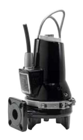
Submersible pump connections 1.5"ANSI | Max Temp 104°F | Cord Length 33' | Cast Iron/NBR | 460 Volts | Explosion Proof Motor | BEP 70 GPM @ 43 FTH
