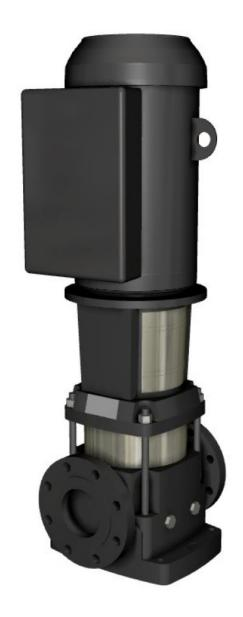
GRUNDFOS VERTICAL CENTRIFUGAL PUMP, WETTED PARTS 316SS, EPDM, MOTOR 3 PHASE 230-460V, CRN64-3-1
