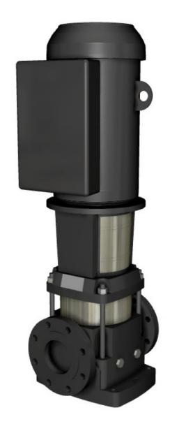
GRUNDFOS VERTICAL CENTRIFUGAL PUMP, WETTED PARTS 316SS, VITON, MOTOR 3 PHASE 230-460V, CRN64-3-2
