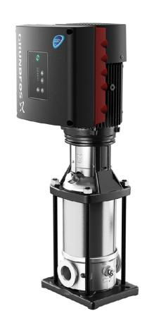
Wetted Material Cast Iron / 304SS-EPDM | Input Volts 440-480 | 1.25" Ansi Flanges | BEP 25 GPM @ 535 FTH
