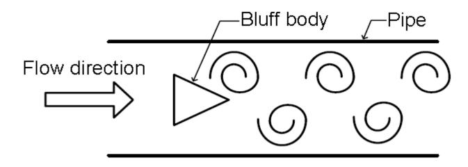
Fig. 2 Operating principle
