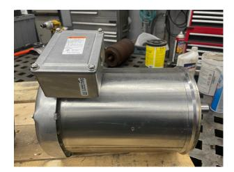
LEESON WASH DOWN, STAINLESS STEEL MOTOR, 5HP, 3600RPM, 184TC FRAME, 208V-230V-460V, 3PHASE
