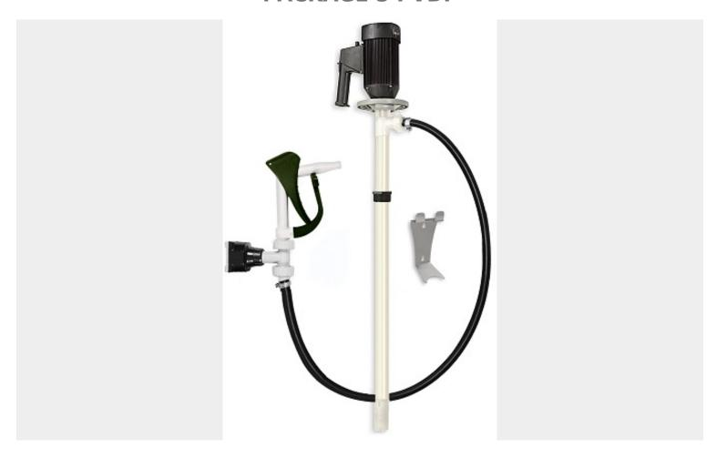
Wetted Material: PVDF, Hastelloy C-276, Carbon Graphite, 6FT Modified Cross-Link Polyethylene Hose, PVDF-Viton Nozzle | 13.5 GPM BASED ON WATER | MAX VISCOSITY 300CPS | MAX TEMP 175°F | Motor Variable Speed | Flow Meter
