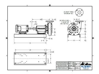
SUMMIT PUMPS FRAME MOUNT 3X4-8 CAST IRON, BRONZE FITTED, MOUNTED ON CAST IRON BASE W/2HP, 1200RPM, 230/460V MOTOR
