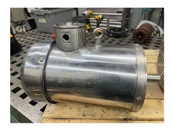
WESTINGHOUSE WASH DOWN, STAINLESS STEEL MOTOR, 5HP, 3600RPM, 184TC FRAME, 230V-460V, 3PHASE
