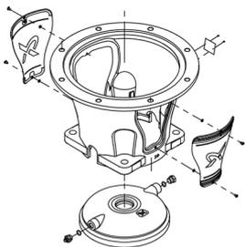
The pump is fitted with a balanced O-ring seal unit with a rigid torque-transmission system. This seal type is assembled in a cartridge unit which makes replacement safe and easy. Due to the balancing, this seal type is suitable for high-pressure applications. The cartridge construction also protects the pump shaft from possible wear from a dynamic O-ring between pump shaft and shaft seal.
