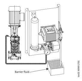
Note: One dosing pump installation can supply several pumps fitted with back-to-back double seal.
