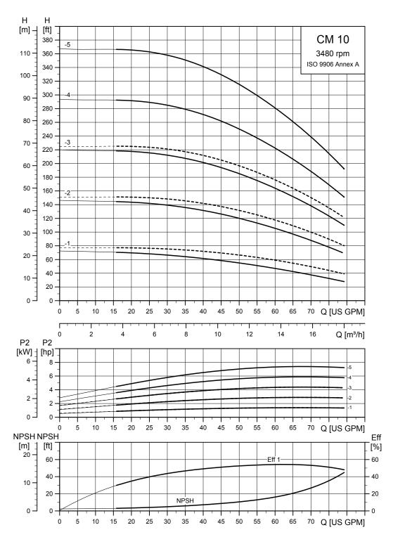
Eff1 = Wire to water efficiency of the pump including motor (see page 39).
