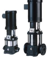
Vertical, multistage centrifugal pump with suction and discharge ports on the same level. The pump head and base are in cast iron - all other wetted parts are in stainless steel (EN 1.4301)
