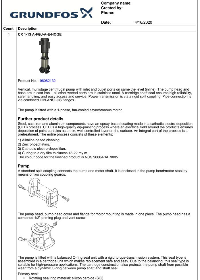
Stationary seat material: silicon carbide (SiC)
