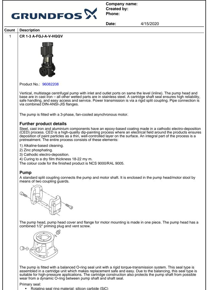
Stationary seat material: silicon carbide (SiC)
