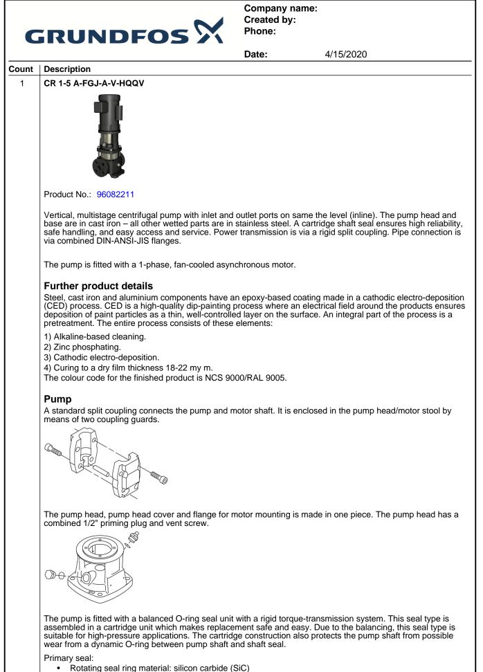
Stationary seat material: silicon carbide (SiC)
