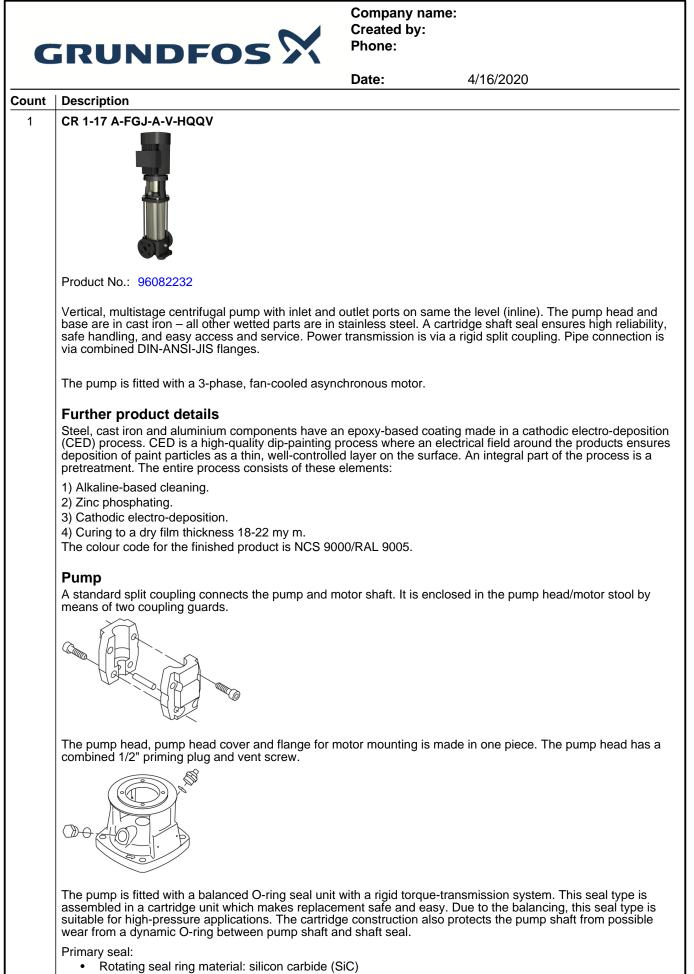
• Stationary seat material: silicon carbide (SiC)
