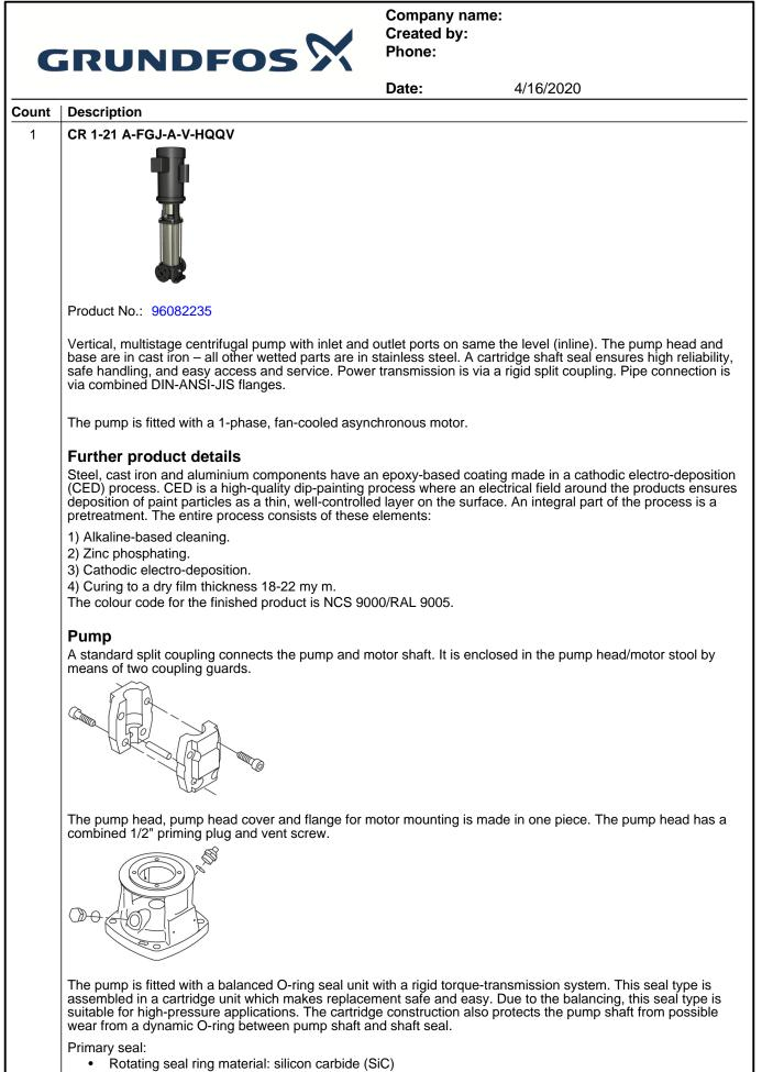
• Stationary seat material: silicon carbide (SiC)
