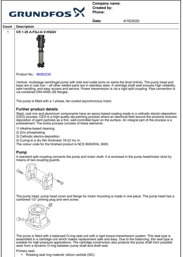
• Stationary seat material: silicon carbide (SiC)
