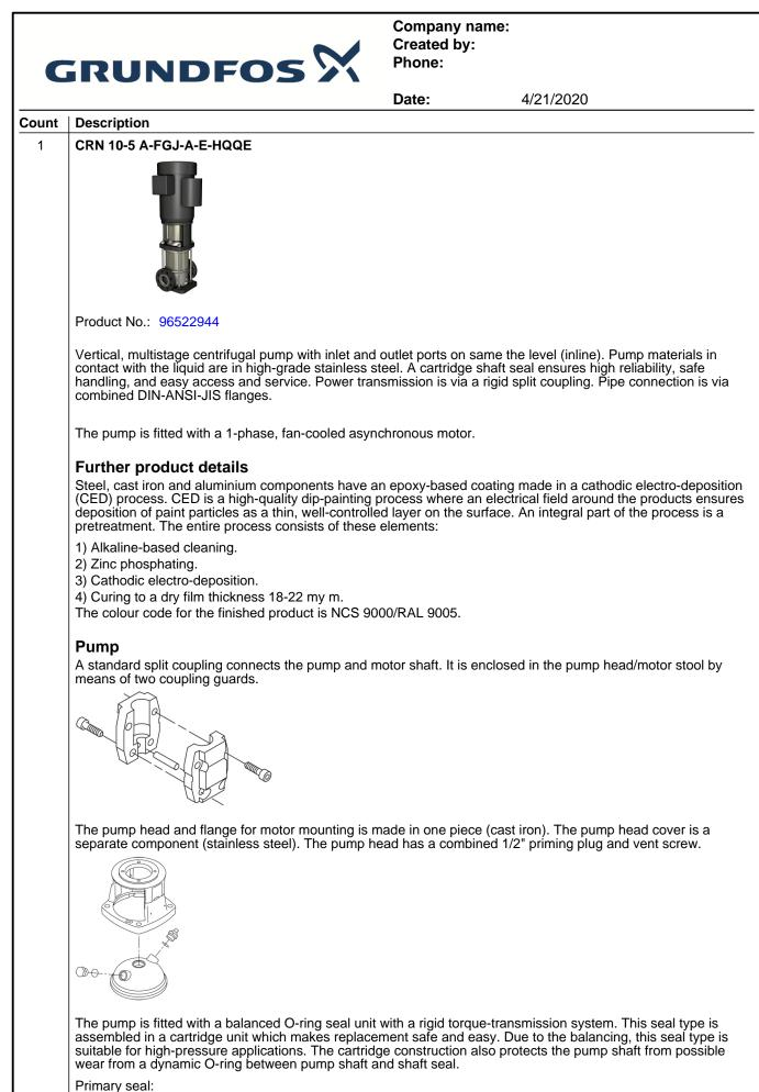
Rotating seal ring material: silicon carbide (SiC)
