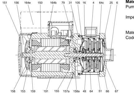
Materials:Pump housing:Stainless steel<br/>AISI 316Impeller:Stainless steel<br/>AISI 316Material code:G<br/>Code for rubber:
