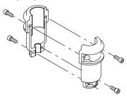
The pump head and flange for motor mounting is made in one piece (cast iron). The pump head cover is a separate component (stainless steel). The pump head has a combined 1/2" priming plug and vent screw.
