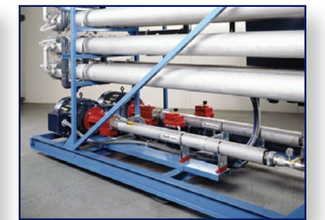
Parallel pumps for higher flow rates
