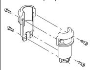
The pump head, pump head cover and flange for motor mounting is made in one piece. The pump head has a combined 1/2" priming plug and vent screw.
