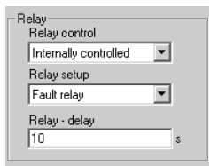
Fig. 25 Signal relay parameters for 1/2 to 10 HP (0.37 to 7.5 KW) pumps
