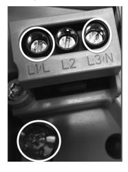
For Three phase **Input Wiring** use L1, L2, L3, and Ground
