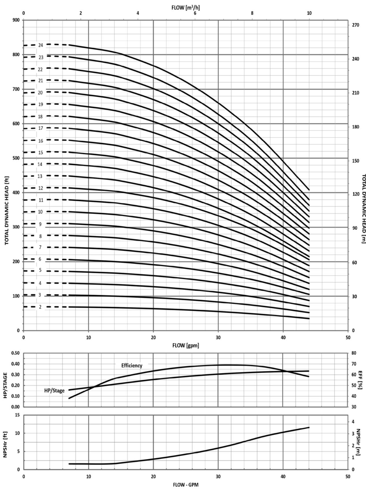
**MINIMUM FLOW RATE: 7 GPM [1.6 m<sup>3</sup>/hr]**
