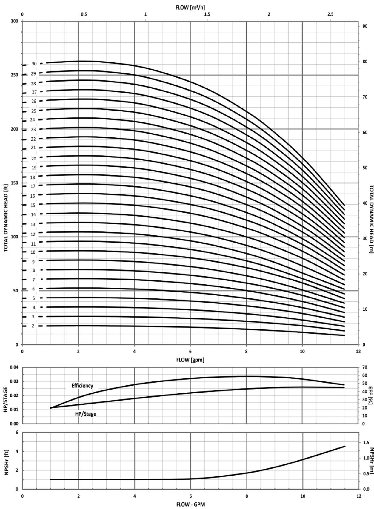
**MINIMUM FLOW RATE: 1 GPM [.24  $\text{m}^3/\text{hr}$ ]**
