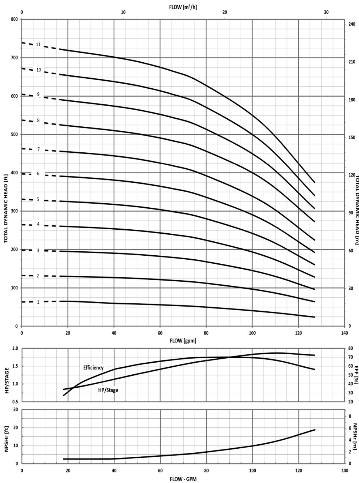
**MINIMUM FLOW RATE: 18 GPM [4.1 m³/hr]**
