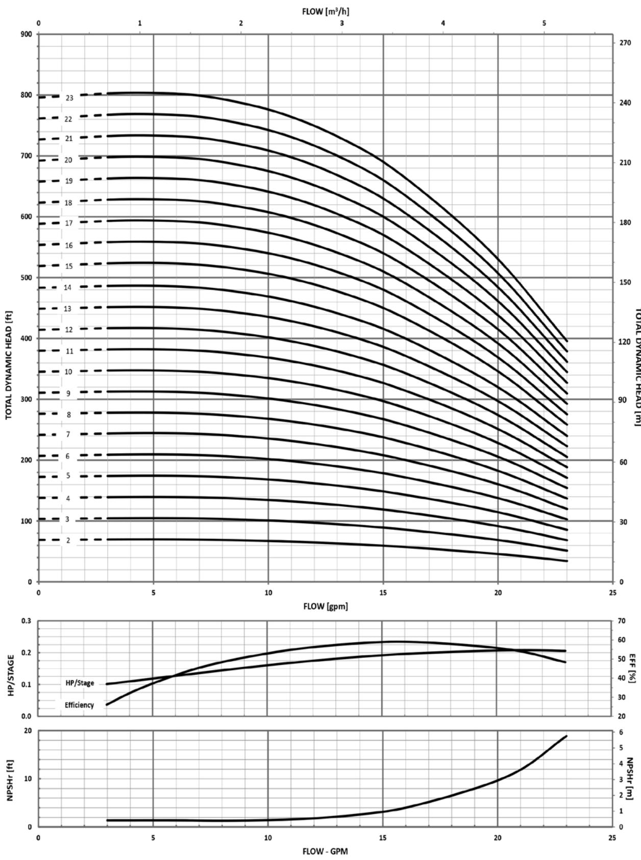
**MINIMUM FLOW RATE: 3 GPM [.68 m<sup>3</sup>/hr]**
