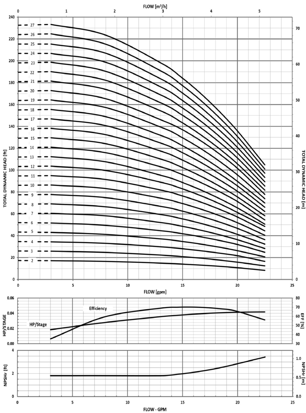
**MINIMUM FLOW RATE: 3 GPM [.7 m³/hr]**
