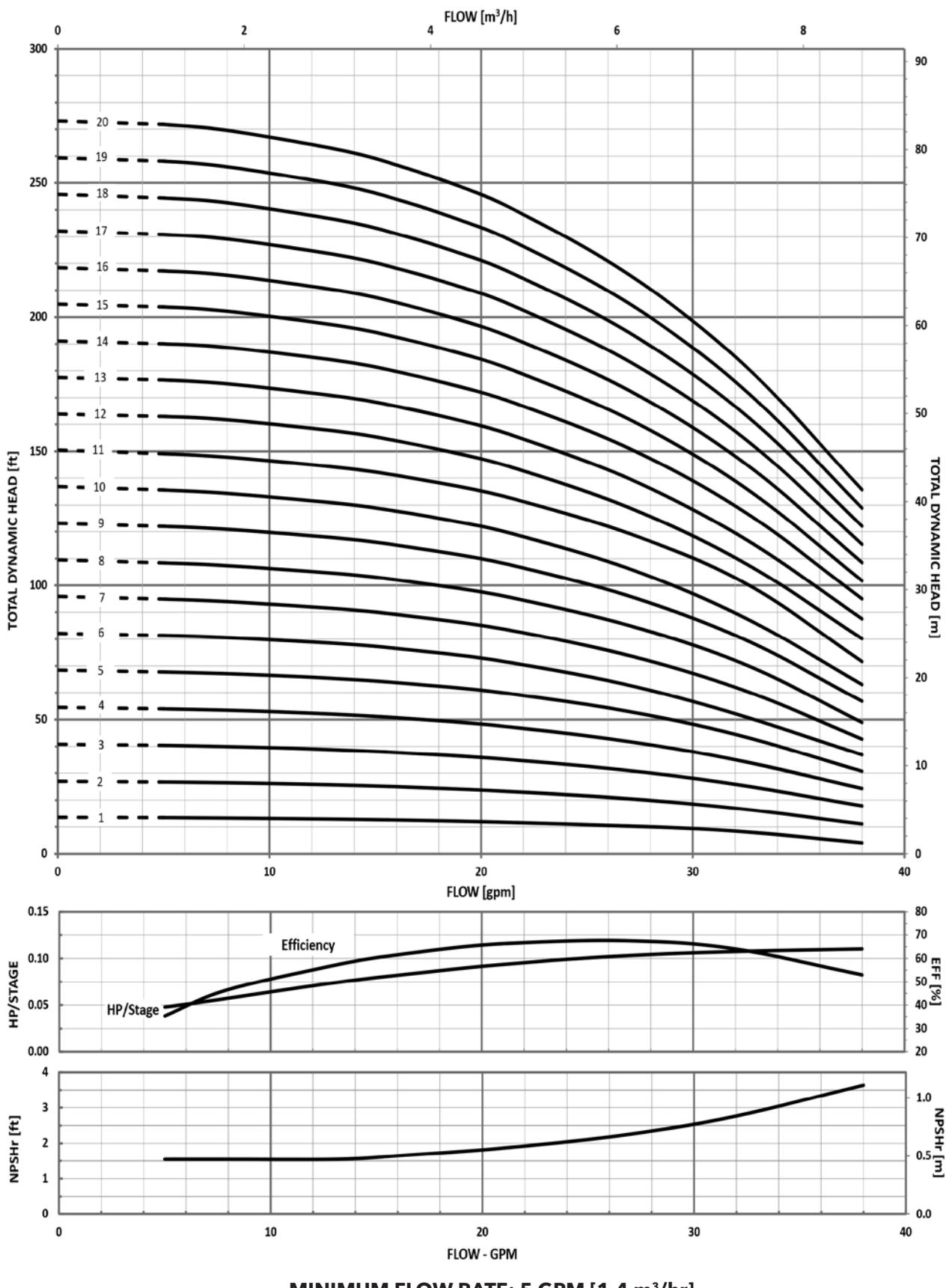
**MINIMUM FLOW RATE: 3 GPM [1.4 L/S]**
