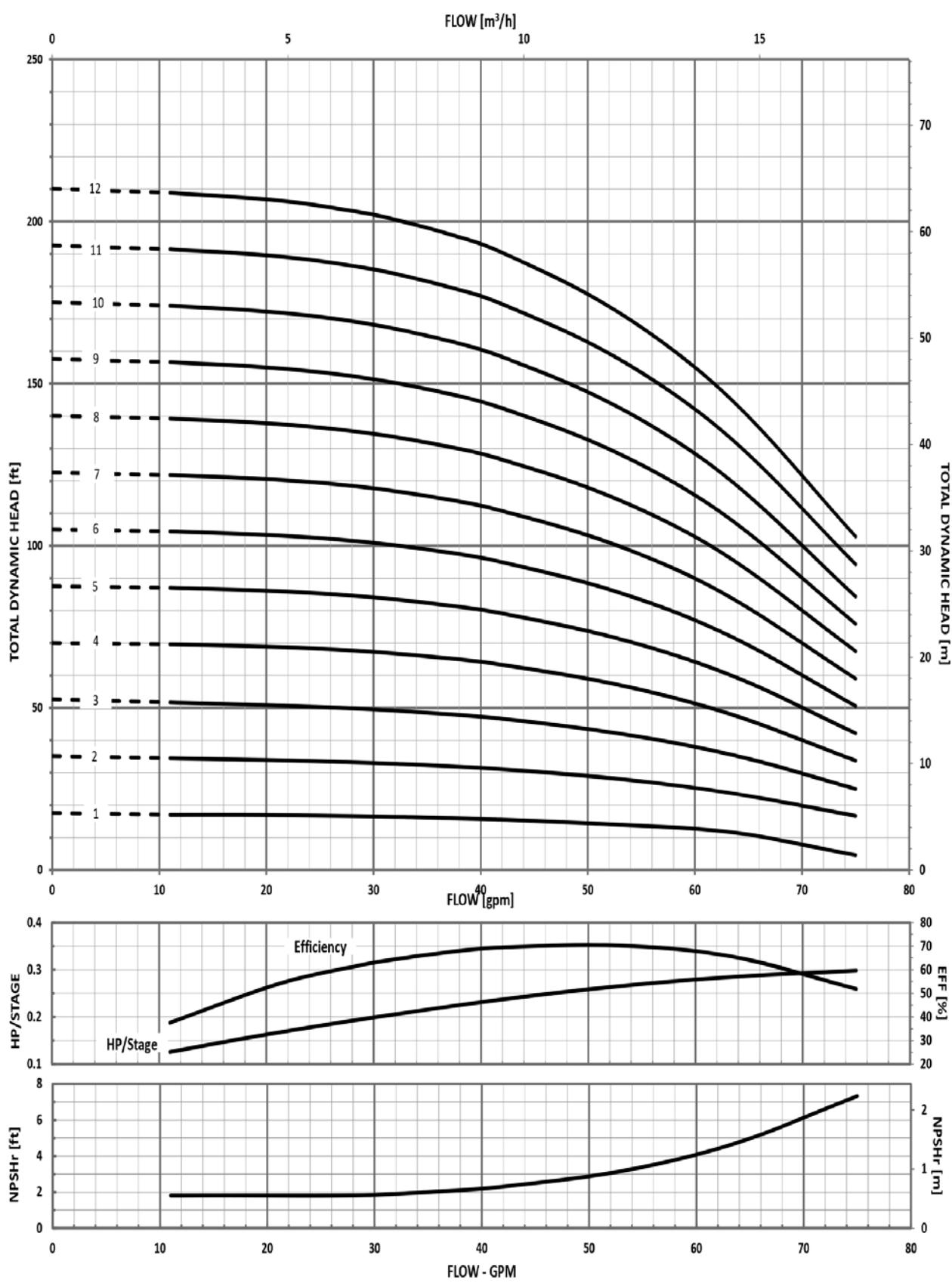
**MINIMUM FLOW RATE: 11 GPM [2.5 m³/hr]**
