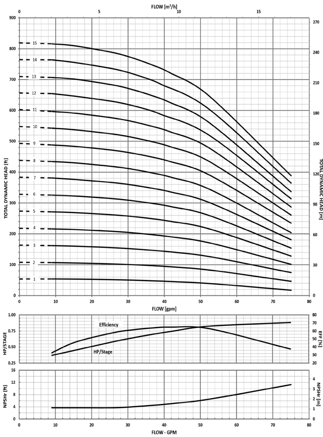
**MINIMUM FLOW RATE: 9 GPM [2 m³/hr]**
