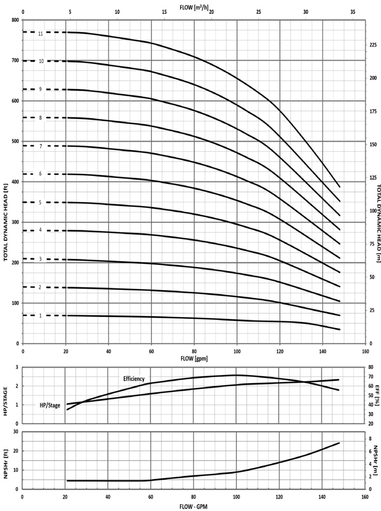
**MINIMUM FLOW RATE: 21 GPM [4.8 m<sup>3</sup>/hr]**
