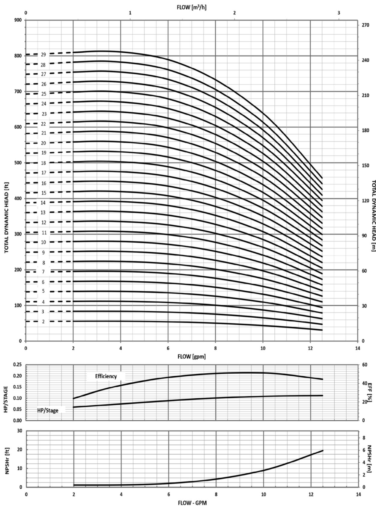
**MINIMUM FLOW RATE: 2 GPM [ $\frac{1}{2}$  m<sup>3</sup>/hr]**
