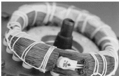
Thermal switch incorporated in winding
