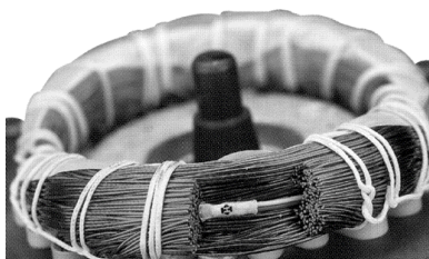
PTC sensor incorporated in winding
