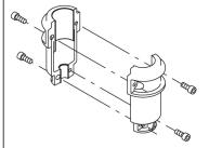
The pump head and flange for motor mounting is made in one piece (cast iron). The pump head cover is a separate component (stainless steel). The pump head has a combined 1/2" priming plug and vent screw.
