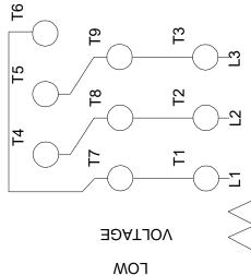
INTERCHANGE ANY TWO LINE WIRES TO REVERSE THE ROTATION
