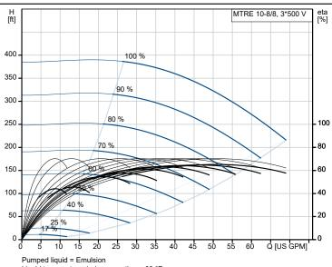
Liquid temperature during operation = 68 °F Density = 62.29 lb/ft³
