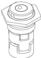
The shaft seal is screwed into the pump head.
