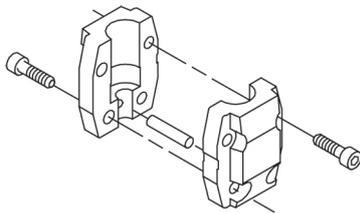
The pump head, pump head cover and flange for motor mounting is made in one piece. The pump head has a combined 1/2" priming plug and vent screw.
