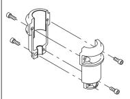
The pump head, pump head cover and flange for motor mounting is made in one piece. The pump head has a combined 1/2" priming plug and vent screw.
