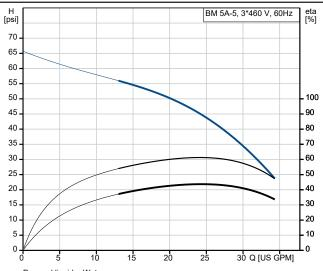
Pumped liquid = Water Liquid temperature during operation = 68 °F Density = 62.29 lb/ft³
