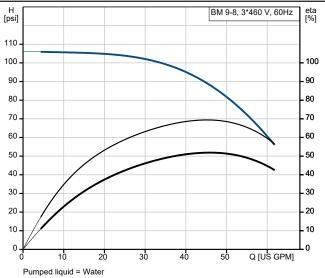
Liquid temperature during operation = 68 °F Density = 62.29 lb/ft³
