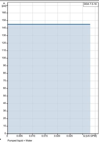
Pumped liquid = Water Liquid temperature during operation = 68 °F Density = 62.29 lb/ft³
