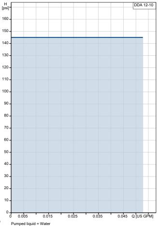
Liquid temperature during operation = 68 °F Density = 62.29 lb/ft³
