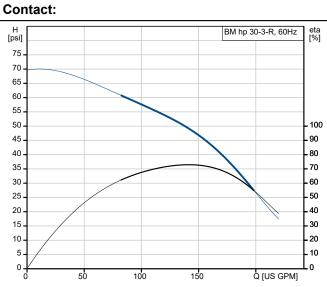
Pumped liquid = Water Liquid temperature during operation = 140 °F Density = 61.35 lb/ft³
