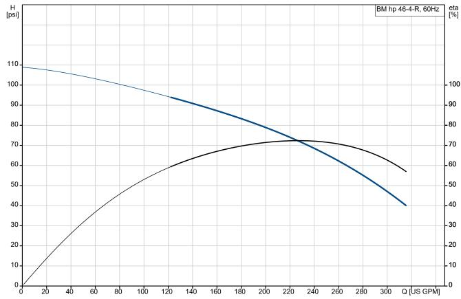
Pumped liquid = Water Liquid temperature during operation = 140 °F
